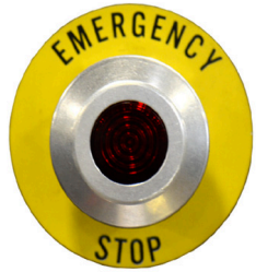
E-Stop in normal run state.
