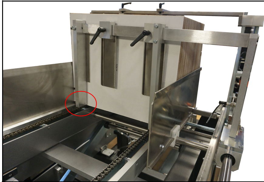
Figure 2-15 - Blank Pusher Assembly
