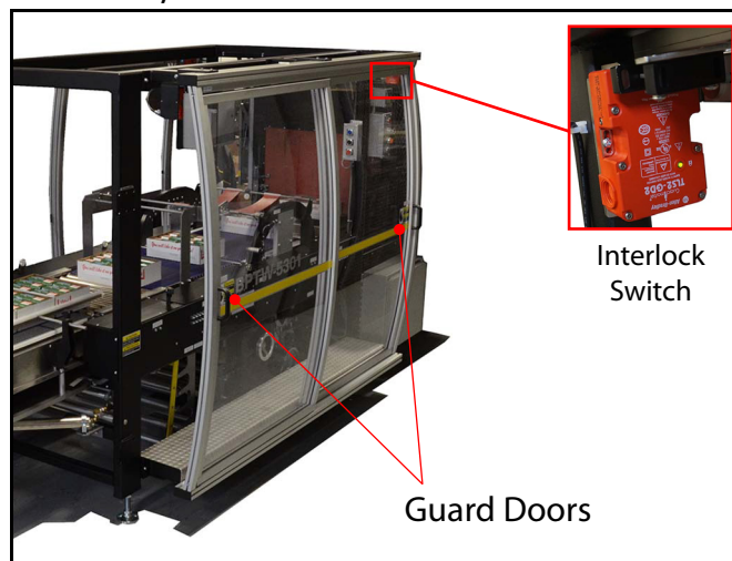
Figure 1-6 - Guard Door & Interlock Switch Example
